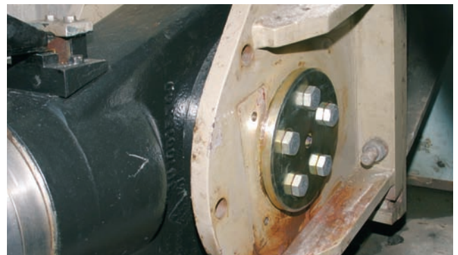
The Expander system is installed. When tightening for the final time, the conical sleeves expand and fill the gap in the mountings on both sides.
